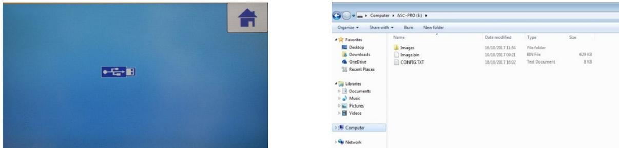
The ASC will now be visible to the external PC as a removable memory device. The root directory of the ASC will contain a file called Image.BIN - this is the firmware file.
