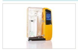
This distillation unit is fully automatic with full microprocessor control. The operator has only to insert the digestion tube and the distillate receiver vessel. The control display is a back-lit LCD with 2 x 16 character lines. Information is entered via the touch sensitive keypad which has numerical characters for entering distillation program parameters, and manual function keys to activate the chemical addition pumps and for programming.
