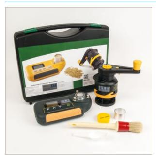
A completely portable unit suited to in-store or field use. Incorporates instant digital-readout of moisture content and automatic temperature compensation for rapid and accurate moisture determinations.
