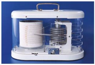
The barograph uses a vacuum capsule to detect changes in atmospheric pressure. The expansion or contraction of the capsule is transferred into a vertical movement which is recorded on the revolving drum.
