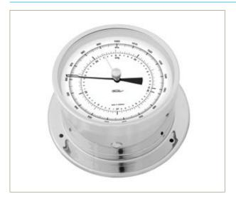
The precision aneroid barometer is used for measuring the absolute atmospheric pressure. The motion of the aneroid barometer is conducted to the axle of the pointer by driving a segment and wheel with an excellent fine finish of the gearing and bearings. This instrument has only got a minimum of idle friction because of the advantageous shape of the bearings and levers. Housing chromed brass with screw on flange diameter 165 mm.
