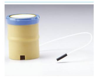
Used to calibrate all types of electrical moisture measuring blocks. The Cup Extractors are (83 mm) 3-1/4 inch overall height by (64 mm) 2-1/2 inch outside diameter and will fit into the 532-120 and 532-100 extractors. Inside cup dimensions are (45 mm) 1-3/4 inch diameter by (51 mm) 2 inch deep.
