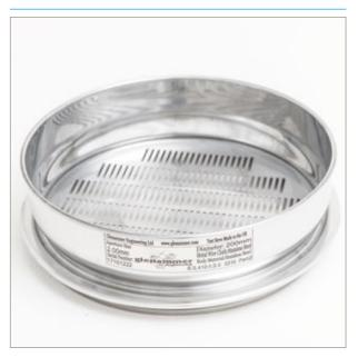
A set of 6 laser-cut stacking grain sieves ensuring the utmost accuracy in grading. The set comprises four sieves with slots 20 mm long x 1.0, 2.0, 2.2, and 3.5 mm wide, made from hard-wearing Stainless Steel plate to BS 6219 and ISO 5223. Also included in the set are two Stainless Steel insect sieves 1.7 mm mesh and 710  $\mu$ m mesh, to aid the control of storage pests such as weevils and mites. A lid and receiver complete the set. Sieves conforming to other standards are available on request.
