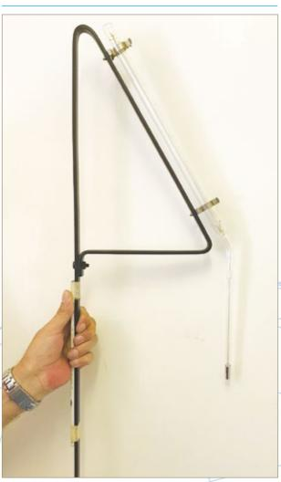
Metal support frame for use with Earth Thermometers.
