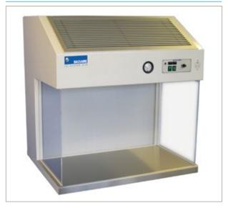
Laminar flow cabinets force sterile air over the work surface and minimise the risk of external contamination and cross-contamination between samples which is essential for sterile inoculation of media during techniques such as tissue culture and micropropagation.
