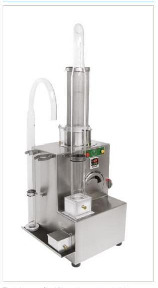
The Laboratory Seed Blower is a precision built laboratory machine designed to separate light and heavy fractions of a great variety of seeds. The blower is equipped with a synchronous motor to ensure uniform RPM and therefore consistent test results. Air flow is regulated with a calibrated vernier gate and adjusted with a calibrated hand wheel for precise adjustments that can be easily repeated. Large tube kit is standard with the Seed Blower.
