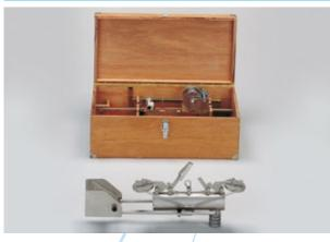
This sampler is designed to be used in a flowing river or stream at any desired depth to 25 metres. The design is such that the open ends through which the water flows can be simultaneously closed, thus retaining the 1250 ml sample which may then be raised to the surface. The accessories include a hand winch, 25 metres of steel wire and a depth meter. The complete set is contained in a wooden transport case with padlock.
