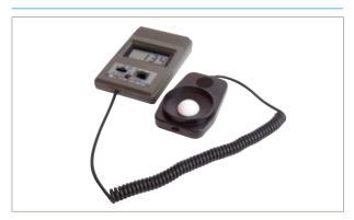
This portable lightmeter is for monitoring illuminance and gives a digital display in Lux. This simple to use instrument has only two controls; a power button and a range switch. It is ideal for field survey work and initial investigations.
