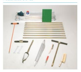
For sampling to a depth of 10 metres. Supplied complete in an aluminium transport case.
