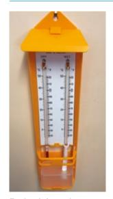
The wet and dry bulb hygrometer is designed for general use and consists of two undivided thermometers mounted on a printed plastic scale. Between the thermometers is a unique slide pointer which allows relative humidity to be easily read. The scale is housed in a plastic case which also holds a reservoir with antifrost device.
