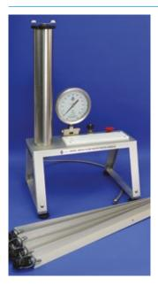
12 inch Pressure Vessel, G4 Specimen Holder, 40 Bar Gauge. Tension in plant xylem can be measured using a plant water status console device. The petiole of a leaf or stem is placed in a rubber grommet so the leaves are inside the pressure chamber and the stem is outside at atmospheric pressure. By pressurising the chamber and watching the point where the sap oozes out of the stem at atmospheric pressure, the two forces are in balance.
