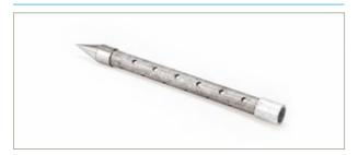
Comprising a porous plastic element. 19 mm diameter x 300 mm long, in a perforated steel tube with hardened steel driving point. Terminates in a 3/4 inch BSP pocket.
