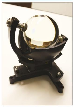
This instrument is used to record the duration of sunshine each day. The sun's rays are focused by a precision glass sphere onto a curved card. The intense heat burns a trace on the card. As the sun moves across the sky, so does the position of the spot across the card. If the sun is obscured by cloud then no trace is made. At the end of the day, the length, less gaps, is proportional to the duration of sunshine.
