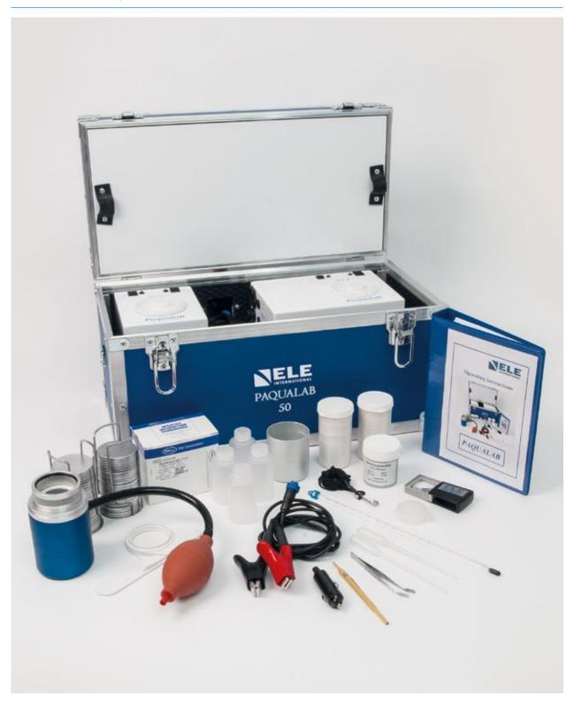
The ELE Paqualab 50 includes two incubators - the standard and universal (each with 2 pre-set temperatures, normally 37°C and 44°C), a membrane filtration unit, microbiological accessories kit, connecting cables and operating manual. All components are housed in a convenient rigid carrying case which can also accommodate a number of electronic meters from the ELE Paqualab range.
