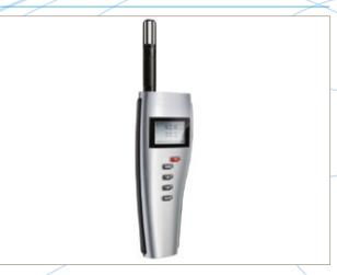
A hand-held instrument that displays relative humidity, temperature and dew point.
