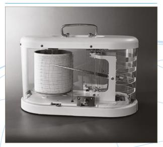
The hygrograph uses hair to detect changes in humidity. The expansion or contraction of the hair is transferred into a vertical movement which is recorded on the revolving drum.
