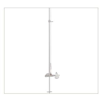
Consisting of current meter, revolution counter, wading rods, base and knob, 3 metre wading cable.
