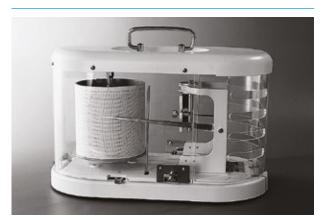
The thermograph uses a bi-metallic element to detect changes in temperature. The expansion or contraction of the element is transferred into a vertical movement which is recorded on the revolving drum.
