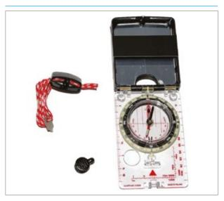
With inclinometer. A folding pocket instrument with sighting mirror in the lid. Used for defining map locations and measuring geological equipment.
