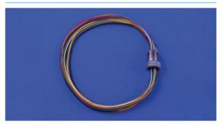
This Stainless Steel 1/4 NPT fitting leads through 10 electrical wires (26 AWG), connected to the fitting with epoxy seal. Handles up to 300 PSI.
