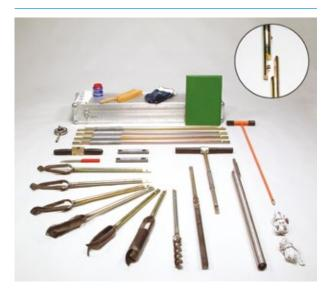
For augering all types of soil above and below the water table to a depth of 5 or 7 metres. Supplied complete in an aluminium transport case with padlock.
