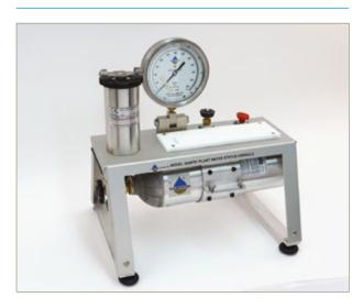
The Plant Water Status Console is supplied with a compressed gas cylinder and connected to a pressure regulator for field operation. The pressure regulator has been set at the factory for the maximum operation pressure of the unit which, for standard units, is 600 psi.
