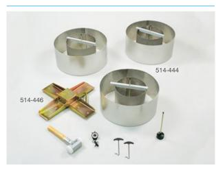
A comprehensive kit used for the determination of infiltration capacity above the water table. Allows synchronous determination of infiltration capacity in triplicate. The components are manufactured from high-quality materials for exhaustive field use.
