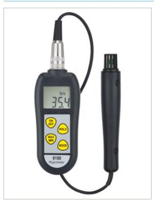
Remote or integral % RH and temperature probe. Displays maximum/minimum humidity or temperature. Optional backlit display. The therma-hygrometer is an easy to use, relative humidity and air temperature measuring instrument. The units measure % RH over the range of 0% to 100% RH with a resolution of 0.1% RH and temperature over the range of -20°C to 70°C with a resolution of 0.1°C. It incorporates a custom LCD, displaying % RH, °C/°F, dew point indication, maximum/minimum and hold.
