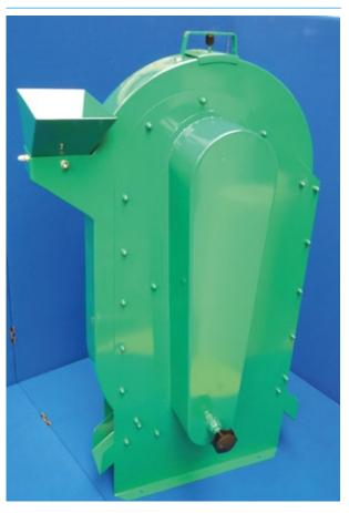
This machine is suitable for pre-cleaning a large number of agricultural products including hulled rice and coffee, wheat, barley and vegetable seeds, by removing light extraneous material such as shrivelled seed, chaff and leaf. Heavy particles including metal and stones can also be eliminated. It consists of an aspirated column with an adjustable flow rate, expansion chamber, air-return ducts and motor driven fan. The fan can easily be removed for cleaning. The unit is bench mounted.
