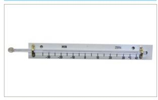
Mounted on plastic scale to match maximum thermometer. Specification as maximum thermometer but recording minimum temperature since last reset, in the range of -35°C to  $+40^{\circ}\text{C} \times 0.5^{\circ}\text{C}$ .
