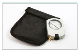
A hand-held precision instrument for determining heights, slopes and vertical angles. The direct sighting device has the peak scale reading visible through the eye piece. Percentage and degree scales permit quick calculation of object heights using a known base line distance. Used by foresters, geologists and surveyors throughout the world.
