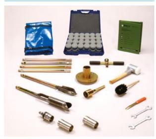
This kit contains the necessary items to sample above and below the water table and comprises the handle and beating head, Edelman auger, a Riverside auger, a closed ring auger and spare cutting shoe, a hammering head and guide cylinder for the rings, a nylon headed hammer, 3 extension rods 500 mm long, 24 numbered sample rings with end caps in an aluminium case, a bent spatula, brush and a carrying bag for all the equipment.
