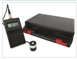
General measurement for human activities. The visible light is that part of the wavelength spectrum received by the human eye. The peak sensitivity is 555 nm for the adapted eye but with 'dark adaption' a peak response is 507 nm. The ranges allow for readings between 0 to 200 K Lux. The sensor has a cosine-corrected head, and the FET input circuitry of the cc measuring and display unit preserves linearity. The unit also incorporates dual slope integration with "auto zero" for A/D conversion.
