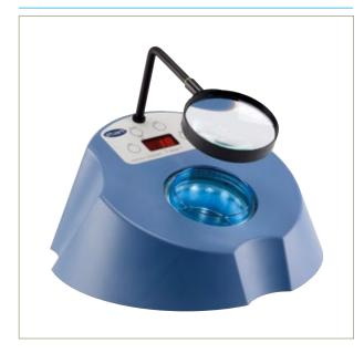
The petri dish is placed on the viewing screen and every time a colony is pressed a count is registered and accompanied by an audible tone. Both the amount of pressure needed to register a count and the volume of the tone are adjustable. The built-in adjustable magnifier enables samples to be examined more easily. For use with up to 100 mm glass or plastic petri dishes.
