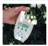
This instrument has been designed to accurately determine the chlorophyll content in plants and crops. Especially useful for improving Nitrogen management programs and is ideal for research and teaching. The ample on-board data storage and hand-held design makes this meter the most field efficient chlorophyll content meter on the market.
