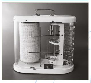
This combination instrument records both temperature and relative humidity on the same chart.
