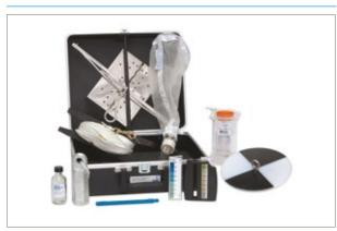
With colour scale, water sampling bottle, plankton net, bottom sampling dredge, sounding lead and calibrated line, 20 metres long marked at 1 and 5 metre intervals, armoured thermometer and Secchi disc (for turbidity check).
