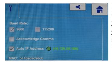
In some situations where DHCP auto IP address is not supported, it is necessary to assign the machine's IP address manually. In this situation deselect the Auto IP Address function and then set up a static IP address from the Calibration Menu, in the Diagnostics & Miscellaneous, Network Set-up section.
