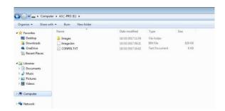
The ASC will now be visible to the external PC as a removable memory device. The root directory of the ASC will contain a file called Image.BIN - this is the firmware file.
