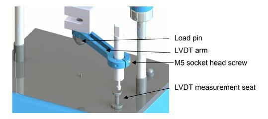
Use a 24 mm spanner (15/16" wrench) to attach the LVDT arm to the load cell with the load pin. Insert the LVDT into the arm and tighten the M5 screw to retain it. The height adjustment may be completed later, see **Motor Drive and Home Position Setup** for details.
