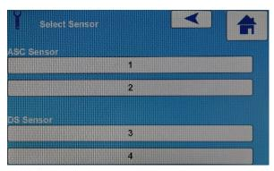
In turn select ASC Sensor 1 and 2. For ASC Sensor 1 and 2 select the DEFAULT option and confirm. The parameters can then be viewed.
