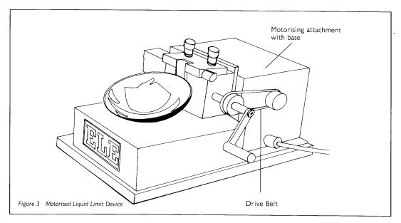
2.2.1 The liquid limit device incorporates a drive assembly with drive and follower pulleys, the latter fitted on the cam shaft of the liquid limit device. A blow counter is included in the motorised version.
