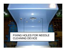
Place the cleaning device on the Vicat machine so that the fixing holes on the appliance are centered with those on the Vicat.
