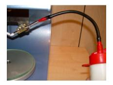
Add three or four drops of oil in the holding devices
