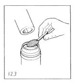
12.4 Holding the membrane only by the edge, place it grid side uppermost centrally on the sintered bronze membrane support. It should only be necessary to remove the aluminium filter funnel momentarily to do this.
