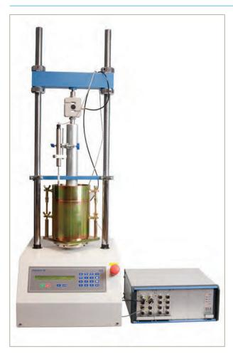
Compact bench mounting load frame designed for performing laboratory CBR, unconfined compression, consolidated drained, consolidated undrained and Marshall Stability tests. Has a variable speed of 0.5 to 50.8 mm per minute and features rapid approach of platen.
