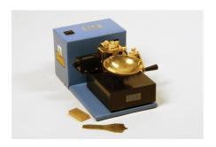
Liquid Limit Device ASTM/ Aashto Hand-Operated W/ Revolution Counter. Supplied Less Grooving Tool.
