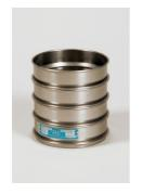
300mm Dia BS Sieve 10.0mm Perforated Plate.
