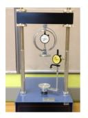
Unconfined Compression Test Accessory Set, Metric Code: 25-3998
