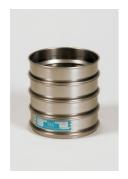
300mm Dia BS Sieve 80mm Perforated Plate
