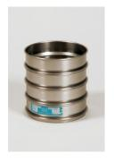
300mm Dia BS Sieve 45.0mm Perforated Plate
