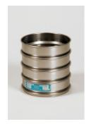
300mm Dia BS Sieve 50.0mm Perforated Plate.
