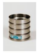
300mm Dia BS Sieve 50.0mm Perforated Plate.
