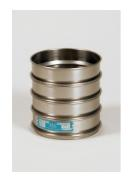
300mm Dia BS Sieve 80mm Perforated Plate
