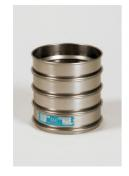
300mm Dia BS Sieve 10.0mm Perforated Plate.
