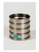
300mm Dia BS Sieve 6.30mm Perforated Plate.
