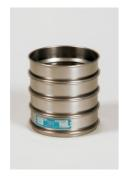
300mm Dia BS Sieve 90.0mm Perforated Plate.
