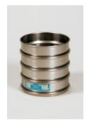
300mm Dia BS Sieve 45.0mm Perforated Plate
