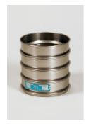
300mm Dia BS Sieve 50.0mm Perforated Plate.
