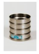
300mm Dia BS Sieve 10.0mm Perforated Plate.
