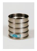
300mm Dia BS Sieve 40.0mm Perforated Plate
