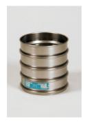
300mm Dia BS Sieve 90.0mm Perforated Plate.
