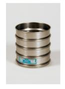
300mm Dia BS Sieve 10.0mm Perforated Plate.
