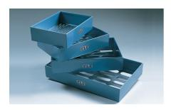
Set of Flakiness Sieves Comprising 1 Ea 4.9mm 7.2mm 10.2mm 14.4mm 19.7mm 26.3mm and 33.9mm
