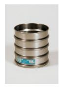
300mm Dia BS Sieve 11.2mm Perforated Plate.
