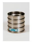
200mm Dia BS Sieve 8.00mm Perforated Plate.
