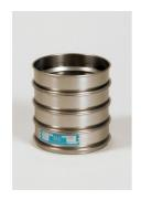
300mm Dia BS Sieve 80mm Perforated Plate
