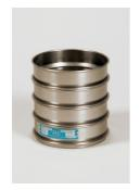
300mm Dia BS Sieve 50.0mm Perforated Plate.
