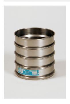
300mm Dia Iso:565 3310/1 Sieve 100 Mic Stainless Steel Mesh. Fitted with Reinforcing Mesh.
