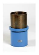
150mm Dia Cylinder Mould 300mm Long.
