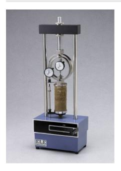
Unconfined Compression Platens. for Use on Ele Load Frames Max Sample Dia 95mm.
