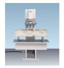
100kN Flexural and Transverse (Flags) Frame. Supplied Without Specimen Bearers and Fitting Kit.
