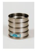
200mm Dia BS Sieve 63.0mm Perforated Plate.
