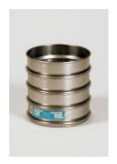
300mm Dia BS Sieve 37.5mm Perforated Plate.
