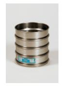
300mm Dia BS Sieve 6.30mm Perforated Plate.
