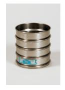
300mm Dia BS Sieve 10.0mm Perforated Plate.
