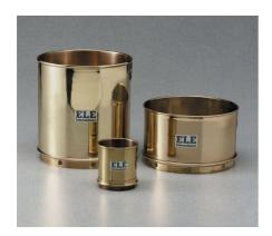
Wet Washing Sieve - 8" diam.  $\times$  8-1/2" h.  $\times$  8" depth to mesh (203  $\times$  216  $\times$  203 mm).
