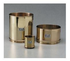
Wet Washing Sieve - 8" diam. x 4-1/2" h. x 4" depth to mesh (203 x 114 x 102 mm).
