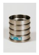
300mm Dia BS Sieve 6.30mm Perforated Plate.
