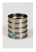
200mm Dia BS Sieve 63.0mm Perforated Plate.
