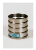
300mm Dia BS Sieve 8.00mm Perforated Plate.
