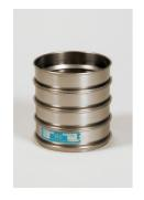
300mm Dia BS Sieve 10.0mm Perforated Plate.
