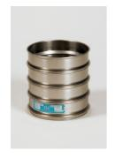
300mm Dia BS Sieve 10.0mm Perforated Plate.
