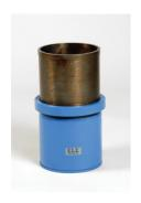
150mm Dia Cylinder Mould 300mm Long.
