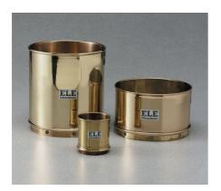
Wet Washing Sieve - 8" diam. x 8-1/2" h. x 8" depth to mesh (203 x 216 x 203 mm).
