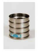
300mm Dia BS Sieve 10.0mm Perforated Plate.
