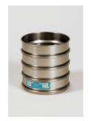
300mm Dia BS Sieve 6.30mm Perforated Plate.
