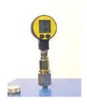
Digital Pressure Gauge 1700 kPa for Use with 26-1800 Series Oil/Water Constant Pressure System.
