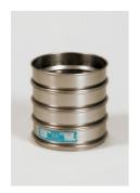
300mm Dia BS Sieve 5.60mm Perforated Plate.
