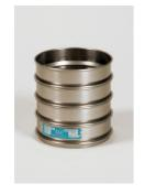
300mm Dia BS Sieve 10.0mm Perforated Plate.
