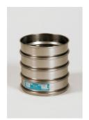
300mm Dia BS Sieve 8.00mm Perforated Plate.
