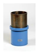
150mm Dia Cylinder Mould 150mm Long.
