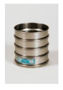
300mm Dia BS Sieve 63.0mm Perforated Plate.
