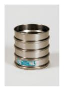
300mm Dia BS Sieve 31.5mm Perforated Plate.
