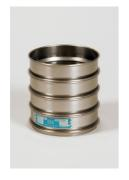
300mm Dia BS Sieve 125mm Perforated Plate.
