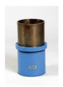
150mm Dia Cylinder Mould 150mm Long.
