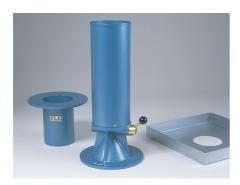
100mm Calibrating Container 100mm ld X 150mm deep with 200mm dia rim.
