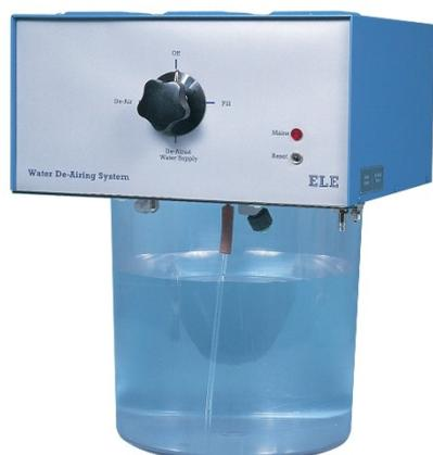
This compact self-contained unit will de-air water quickly and efficiently down to levels of dissolved oxygen acceptable for geotechnical test methods. Air is removed from the water by a vacuum system, which continuously circulates the water in the tank. The unit is supplied with a clear water container, which will hold a maximum of 15 litres of water. Input and output lines are formed using standard 6 mm tube connectors.
