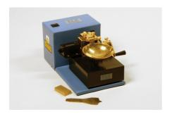
Liquid Limit Device ASTM/ Aashto Hand-Operated W/ Revolution Counter. Supplied Less Grooving Tool.
