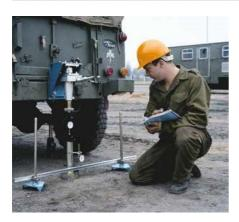
Land Rover Bracket to Attach EL29-200 Jack. for Land Rovers Models 90 & 110 From 1983 Onwards.
