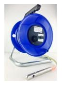
Water level indicator (dipmeter) with audio and light indicator 200 m
