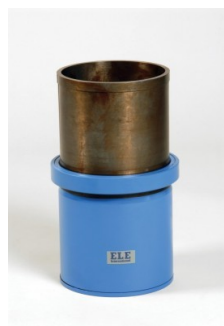
150mm Dia Cylinder Mould 150mm Long.
