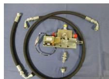
**100 kN Flexural Fitting Kit ADR Auto for 220 - 240 V AC, 60 Hz, 1 ph**
