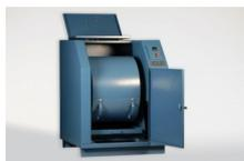
**Los Angeles Abrasion Machine with CE Safety Cabinet W/ Microswitches. 220-240V 60Hz 1Ph.**
