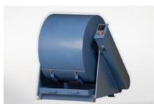
**Los Angeles Abrasion Machine Meets ASTM and European Standards. 220-240V 50Hz 1Ph.**
