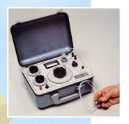
**513-135 Salinity Bridge measuring Instrument.** This instrument provides a method for accurate measurement of salinity in soil solutions without continuous disturbance to the soil profile. The sensor consists of a pair of electrodes embedded in a porous ceramic element. The water saturating the element remains in chemical equilibrium with the soil. The sensor is spring loaded to maintain hydraulic contact between the sensor and the soil.
