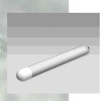
**450-060 Soil water sampler.** Instrument consists of a sample collection tube and porous ceramic cup, through which the soil water passes. The sampler is installed at the desired depth and a vacuum is created in the sample tube to enable the collection of soil water. Operation of the sampler requires the universal extraction kit (450-066).
