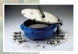
Pressure Plate Extraction Systems. Soilmoisture's pressure plate extraction equipment has been developed to determine soil water retention and suctions from 0.1 to 15 bar. Positive air pressure is used to drive water from the soil matrix to determine; available water capacity, water retentivity, hydraulic conductivity and field capacity. Systems can be assembled to suit the users individual needs.
