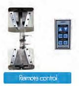
Using its open type hydraulic chuck system, fitting of test samples is convenient by the operation of remote control. The open type hydraulic chuck system enables easy fitting of the test sample and prevent slipping thus provide safety to the user.
