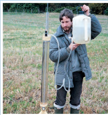
2) Install Permeameter and fill with water
