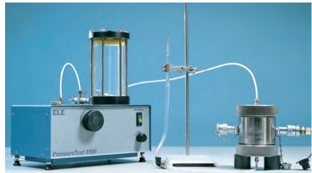
Permeability Test with Pressure Test 3500 Pressure System.
