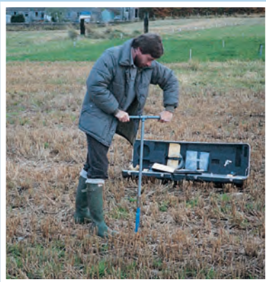
1) Auger and prepare hole
