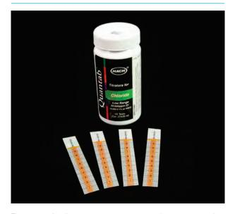
Type 1175 titration range 0.005% to 0.1% (30 to 600 ppm) NaCl. Pack of 40.
