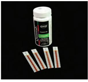
Type 1176 titration range 0.05 % to 1% (300 to 6000 ppm) NaCl. Pack of 40.
