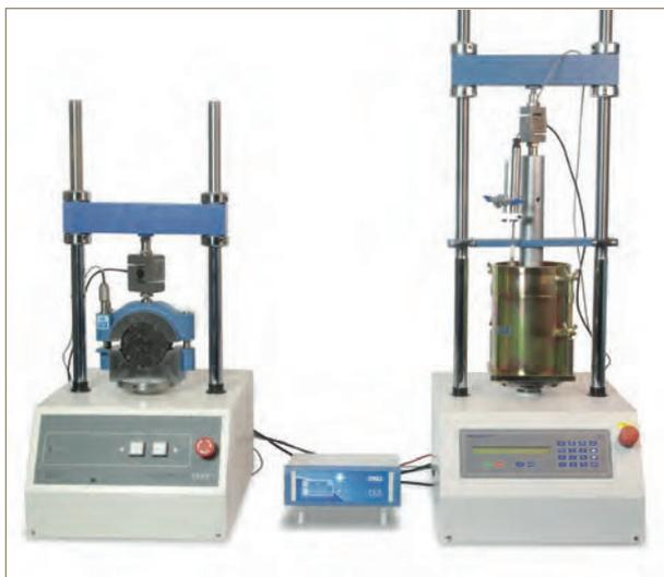
The Data System Unit (DSU) is a versatile instrument designed to accommodate the general logging requirements of geotechnical and materials testing engineers. Its intelligent interface allows the user to work with a range of different sensors.
