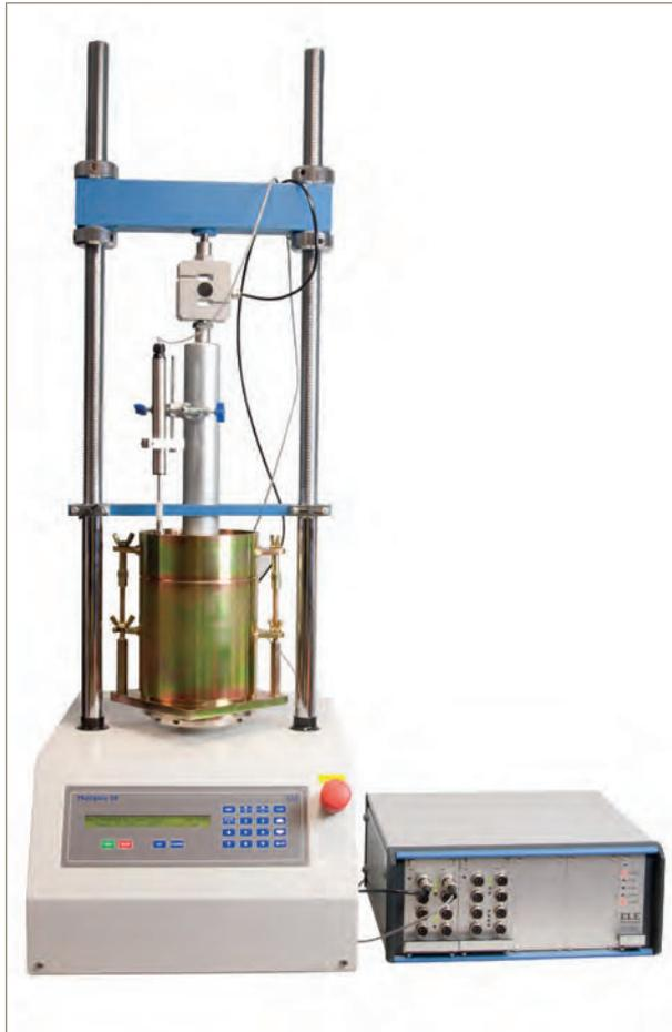
Compact bench mounting load frame designed for performing laboratory CBR, unconfined compression, consolidated drained, consolidated undrained and Marshall Stability tests. Has a variable speed of 0.5 to 50.8 mm per minute and features rapid approach of platen.
