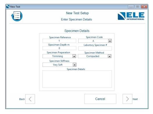
**Note:** the Specimen Stiffness drop down menu is only valid for the Auto Soil Consolidation test, for Manual One-Dimensional Soil Consolidation tests this is not taken into consideration.
