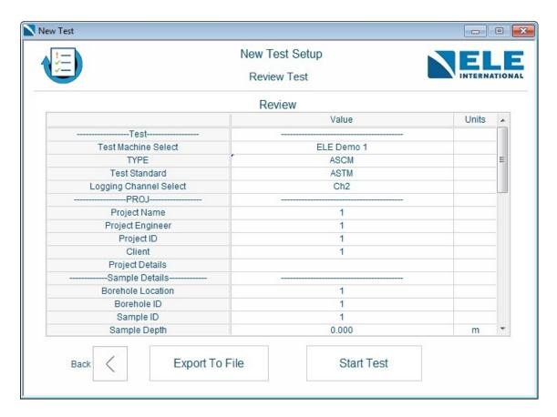
This Test setup can be saved to a file for future use by clicking 'Export To File'. The test setup will be saved with the Project Name - Project ID-SP Ref-SP Code.atf file at location:-
