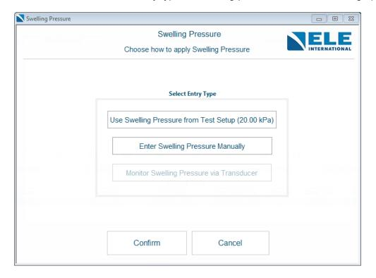
Swelling pressure value should be added manually to each stage pressure if selected. Once complete, a message will pop up to start the test.
