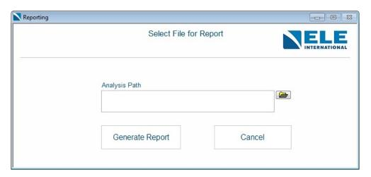
Select the analysed file from the list of completed tests and click on the Generate Report button to create a report.
