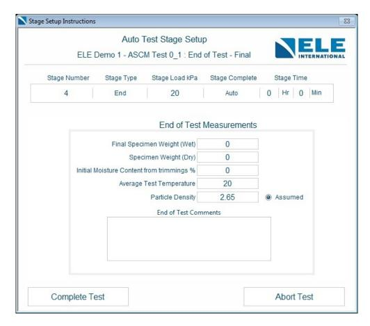
The user will be asked to enter the End of Test Measurements. Once complete, click on the 'Complete Test' button to finish the test.
