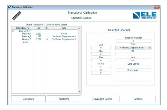
To add a new transducer calibration setting, click on the Calibrate button.
