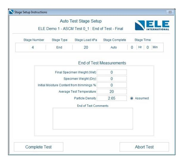
The user will be asked to enter End of Test Measurements. Once complete, click on the 'Complete Test' button to finish the test.
