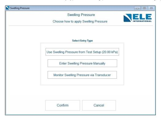
Monitor Swelling Pressure via Transducer will allow the user to carry out a free swelling test.
