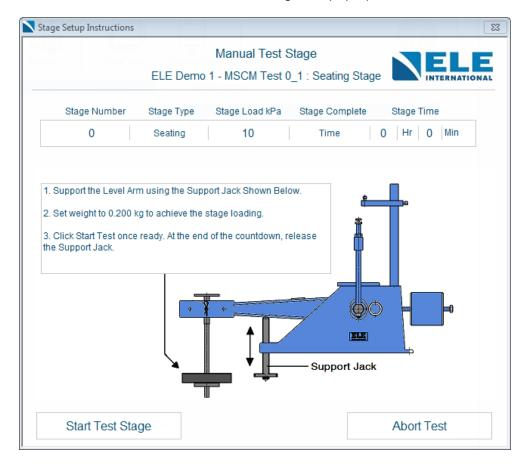
Apply the seating load, click on the Start Test Stage and the user will be prompted to choose options for entering the swelling pressure if, during the test set up, the Specimen Moisture is selected as Inundated.
