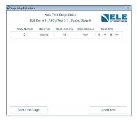
Click on the Start Test Stage to start the test. Once the seating load is reached, the user will be prompted to choose options for entering the swelling pressure if, during the test setup, Specimen Moisture has been set as Inundated.
