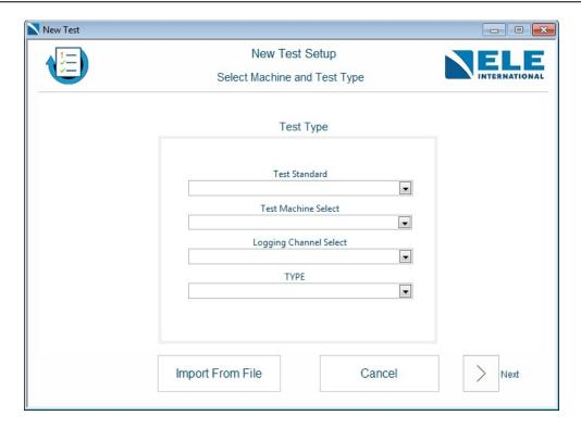
On this screen, select the machine and enter the test details - Test Standard, Logging Channel and Test Type.
