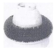
This filter brush is fixed to an aluminium ring, which can put the appliance into the water reservoir (see figure above). The electric flex of the appliance must be drawn through the ring. The air required by the unit is then forced to pass through the filter brush, which traps the fibrous dust. This prevents the accumulation of dirt in the unit to a large extent, and maintenance can be carried out at longer intervals.
