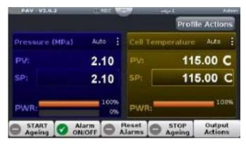
Once the PAV has reached the set point, wait for 20 minutes to condition the pan holder.
